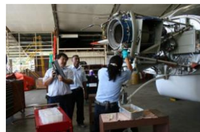
The caravan crew replacing some damaged engine
