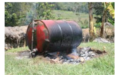
Hot water heater village-style
