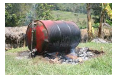
Hot water heater village-style
