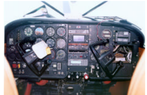
The new radio stack Hugo installed in MAB
